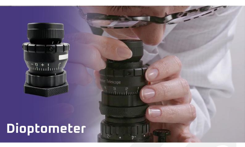
A dioptometer is an optical instrument primarily used to measuring the power of lenses in diopters. It works by determining the focal length of a lens or the eye's refractive error in diopters, which is a unit of measurement representing the optical power of a lens.
